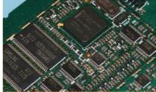
Figure 2: Surface mount components.
